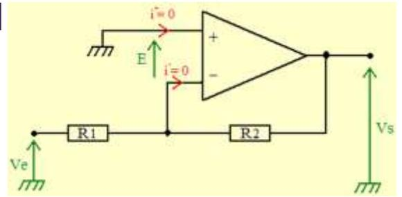
$$V_S = V_E \times \left( -\frac{R_2}{R_1} \right)$$
