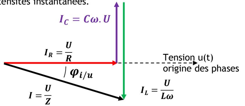
$$\frac{1}{Z_{RLC}} = \sqrt{\frac{1}{R^2} + \left(C\omega - \frac{1}{L\omega}\right)^2} ; \tan \varphi_{i/u} = R \times \left(C\omega - \frac{1}{L\omega}\right)$$
